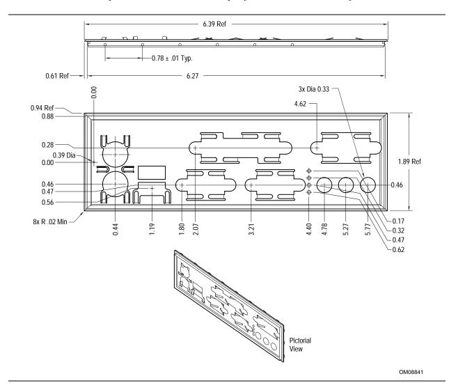
Figure 16. I/O Shield Dimensions
